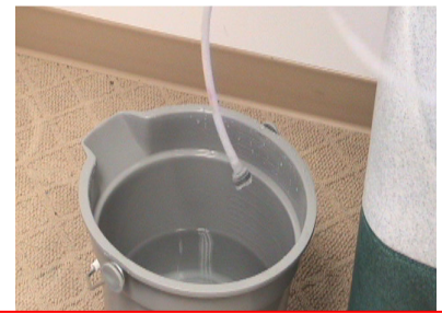
Place Chemical Feed Hose into Rinse Solution
